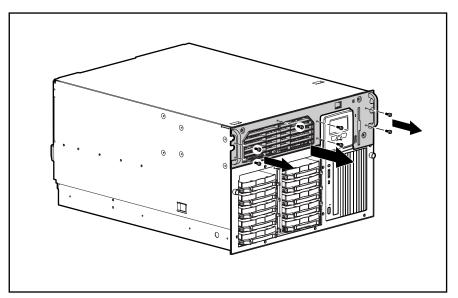
Figure 2-5. Removing the rack-mount bezel
